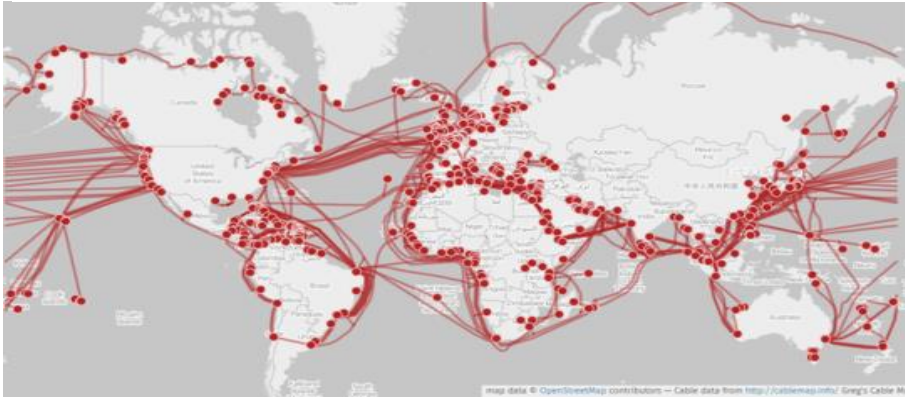
Figure 6. Routing of prominent undersea cables that serve as the physical infrastructure of the Internet
